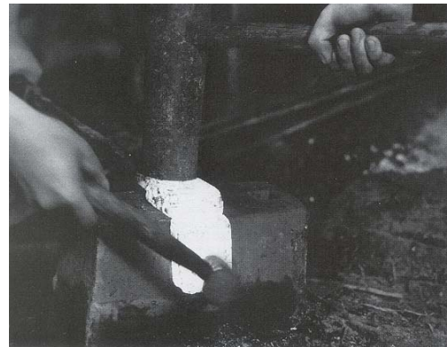
Figure 16: Bar of kawagane steel being folded. The metal is being bent to a 90 degree angle. [2]
