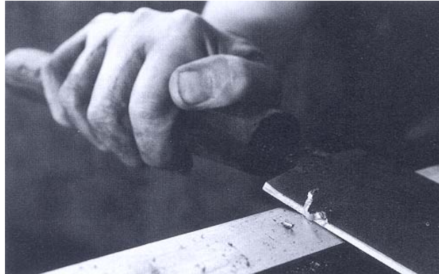
Figure 27: The removal of irregularities from the surface of the metal. Note the drawknife or sen . [2]
