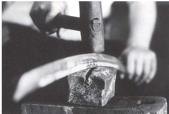
Figure 33: Correction of the curvature of a katana blade through the sorinaoshi . Causing the metal to expand with a heated copper ingot increases the curvature. [2]
