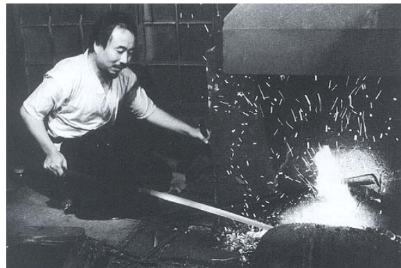
Figure 31: The sword smith draws the blade through the forge to homogenize the temperature of the metal. [2]
