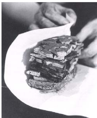
Figure 14: A stack of tamahagane steel being wrapped in rice paper to maintain its form during heating. [2]
