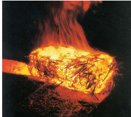
Figure 18: Heated bar of kawagane steel coated in rice straw ash. [2]
