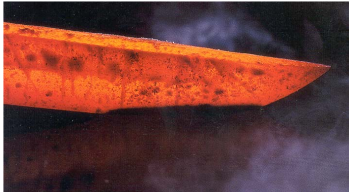
Figure 32: Quenching of the heated blade. This process will cause the formation of hard martensite in the cutting edge. [2]
