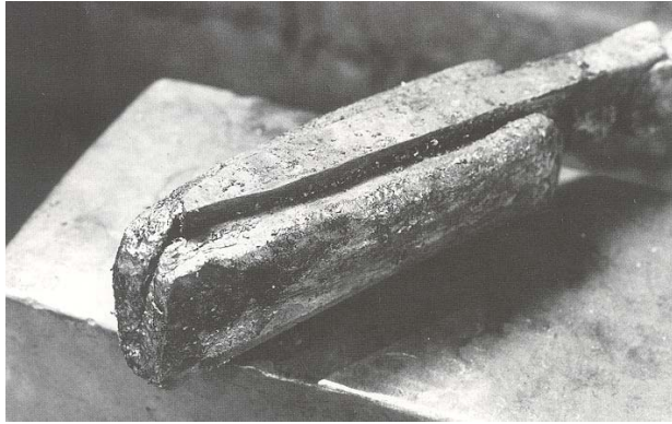
Figure 22: Welded bar of steel from tsukurikomi process. Kobuse-gitae style. Note how the shingane core rests in a jacket of kawagane . [2]
