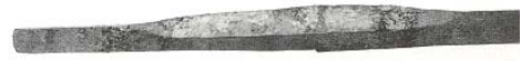
Figure 25: A 6” section of a sunobe . The cutting edge is being drawn out. Note that only a 6” section is worked at a time. [2]
