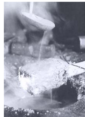
Figure 15: Clay slurry is applied to a heated stack of tamahagane to provide insulation during heating. [2]
