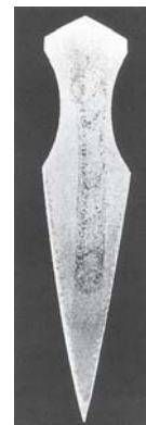
Figure 25: Cross-section of a katana blade. Kobuse-gitae style tsukurikomi . Note the difference between the soft, dark core and the hard, bright sections of metal. [2]
