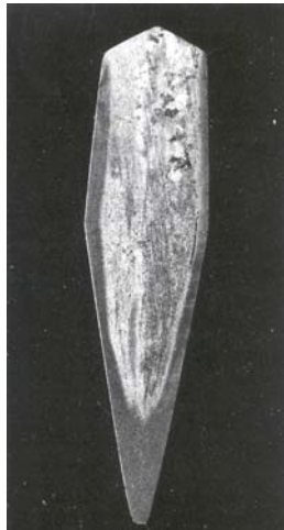
Figure 9: Cross-section of a katana blade. [6]
