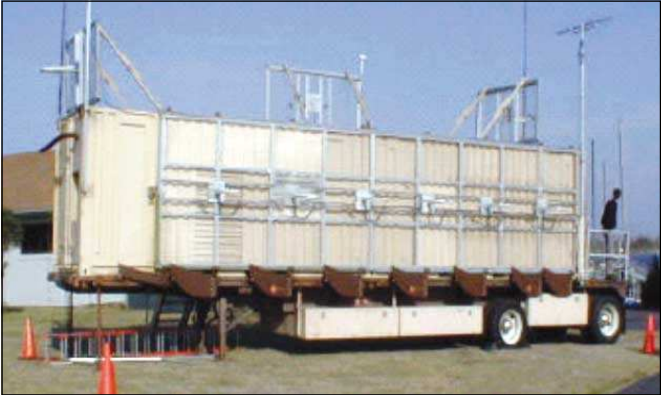
Silent Sentry Passive Radar
