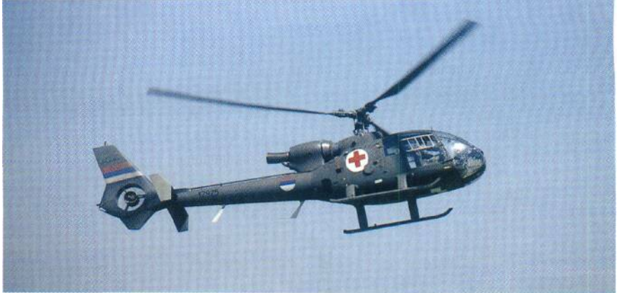
The favoured variant of the ubiquitous Gazelle is the SA-342L because of its higher power rating over the basic SA-342H. Note the 'helicopter' variant of the national markings on this example, marked with a red cross. ALEKSANDAR RADIC
