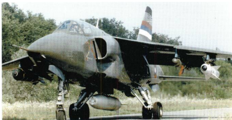
Above: J-22NS Orao (Eagle), serial 25173, displays a non-typical weapon load for the camera. Slung underneath (from l to r) are: Hunting BL-755 cluster bomb dispenser, Plab-350 Napalm munition, Matra Durandal runway penetrator and Hughes AGM-65B Maverick. Insert: The official RV i PVO VRS insignia. RV i PVO VRS
