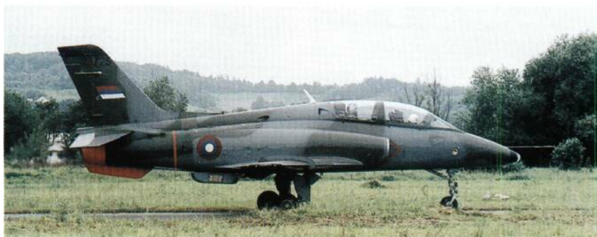
The sole example of the Republic of Srpska's SOKO G-4 Super Caleb is used primarily for training Orao pilots. Note the Yugoslav-designed flare pack mounted under the rear fuselage. ALEKSANDAR RADIC
