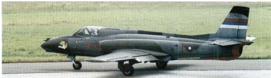
The Jastreb does not have tip tanks fitted for the light attack role, since the short-range missions flown by the type place greater emphasis on manoeuvrability than on endurance. The emblem on the nose of this Jastreb is 'the Lynx from Vrbas' (Vrbas being the river running through Banja Luka) and was inherited from the former Yugoslav Air Force 238 Fighter-Bomber Squadron. ALEKSANDAR RADIC
