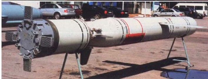
The first-stage booster of the 3M54E1 missile
