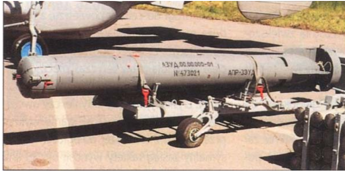
The APR-3ME rocket torpedo, the payload of the 91RE1 missile
