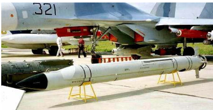
The 3M51E on display in 1996, by Novator NPO, in front of a Su-27IB Flanker. The scoop for the turbojet is visible to the rear of the missile.
