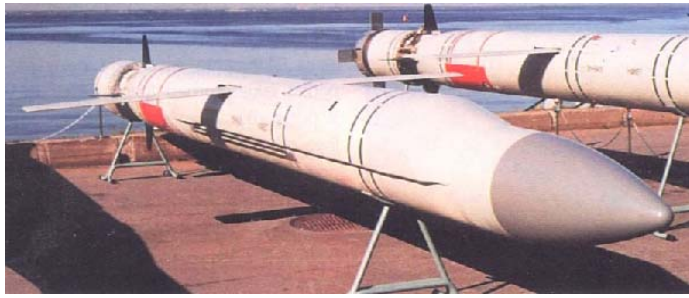
The supersonic 3M51E, with wings extended. The missile also goes by the designation, ASM-MS.
