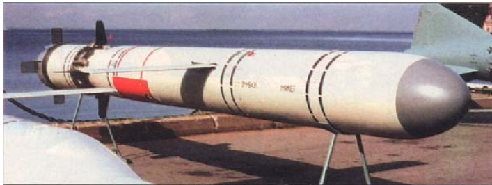
The subsonic 3M54E1's two stage motor gives it a long reach of 300 km
