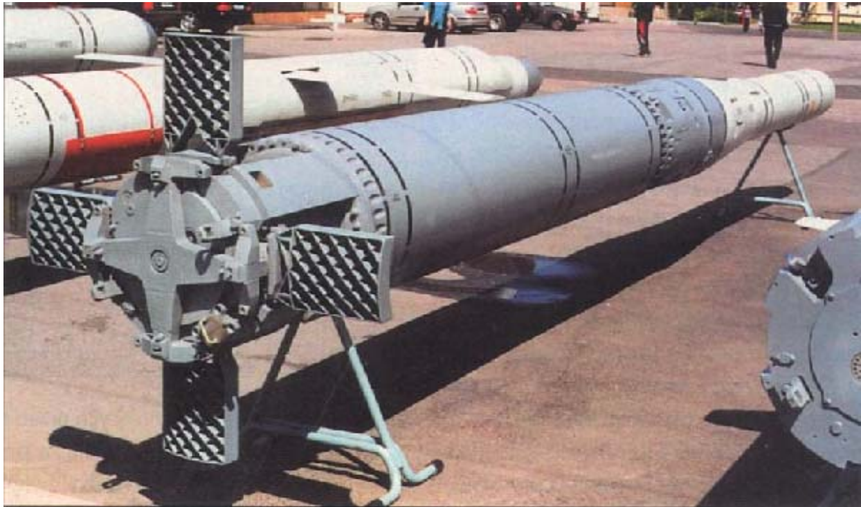
The first-stage booster of the 91RE1 missile
