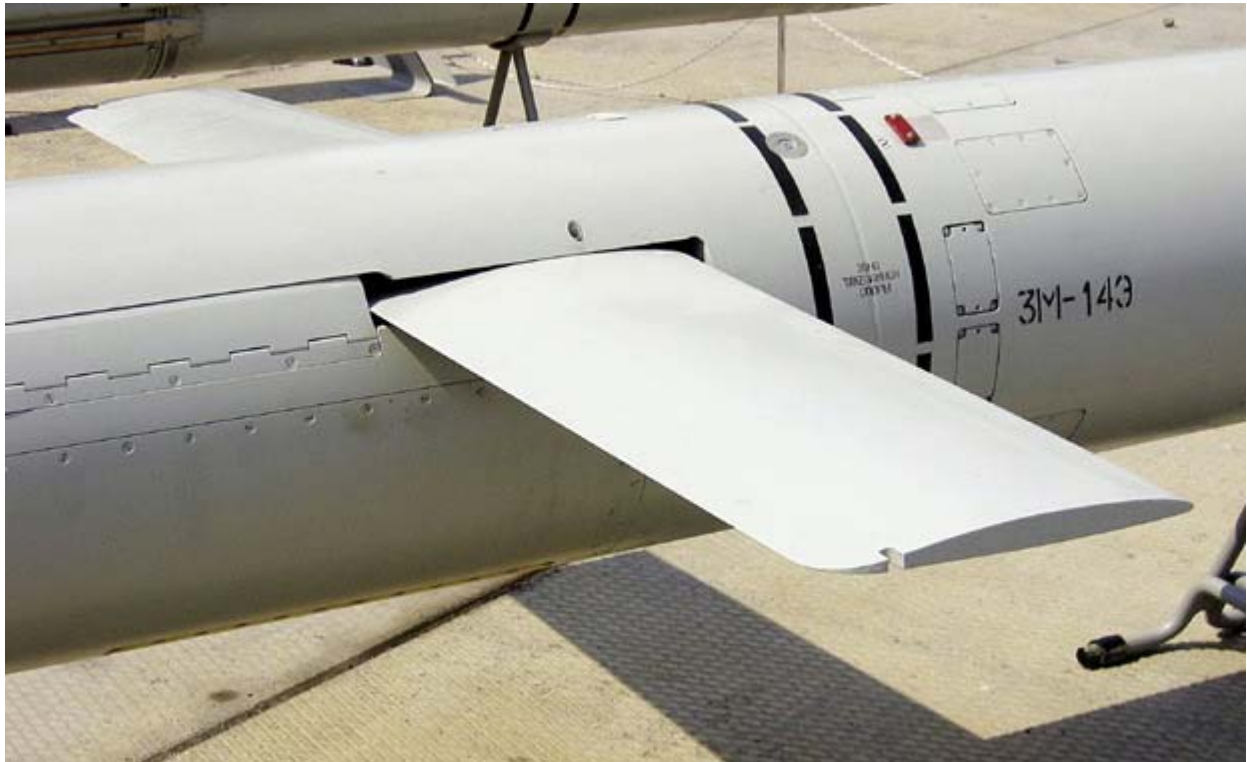
A close up shot of the 3M-14E's missile fins which it uses to maintain attitude control during flight.
