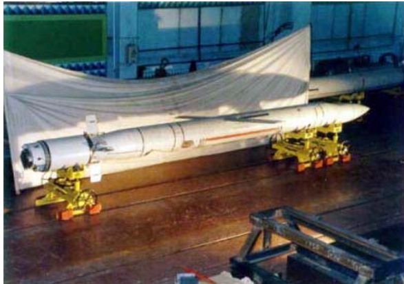
The pointed nose of the supersonic rocket, which forms the payload of the deadly 3M54E AShM, protrudes from the front of the complete missile
